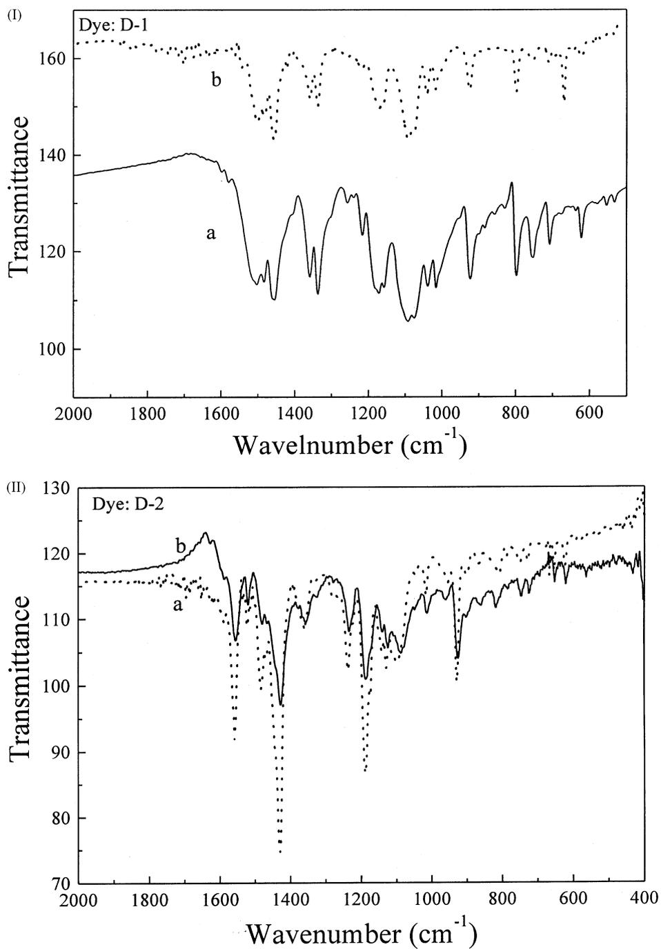
Fig. 2. IR spectra of the powder (a) and thin film (b) deposited from tetrafluoro-propanol: (I) D-1; (II) D-2.
