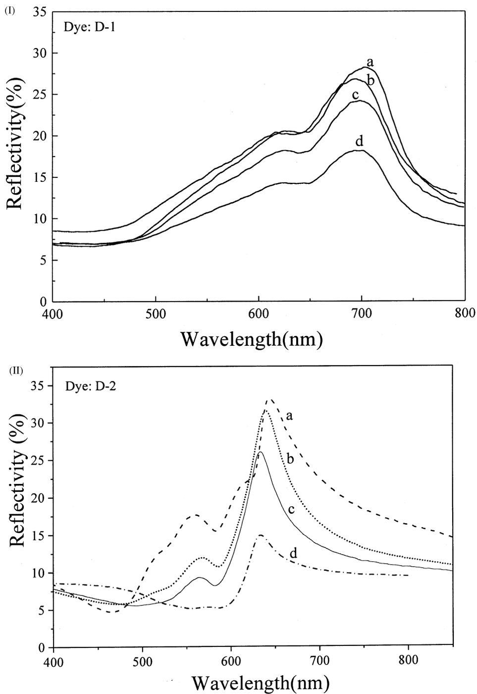
Fig. 3. The reflection of D-1 and D-2 films deposited from different pure solvents: (a) chloroform; (b) tetrafluoro-propanol; (c) diacetone alcohol; (d) methanol: (I) D-1; (II) D-2.
