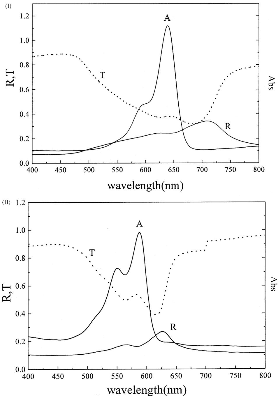
Fig. 1. Absorption spectra of dyes in methanol and the transmittance and reflection of dye film: (I) D-1; (II) D-2.
