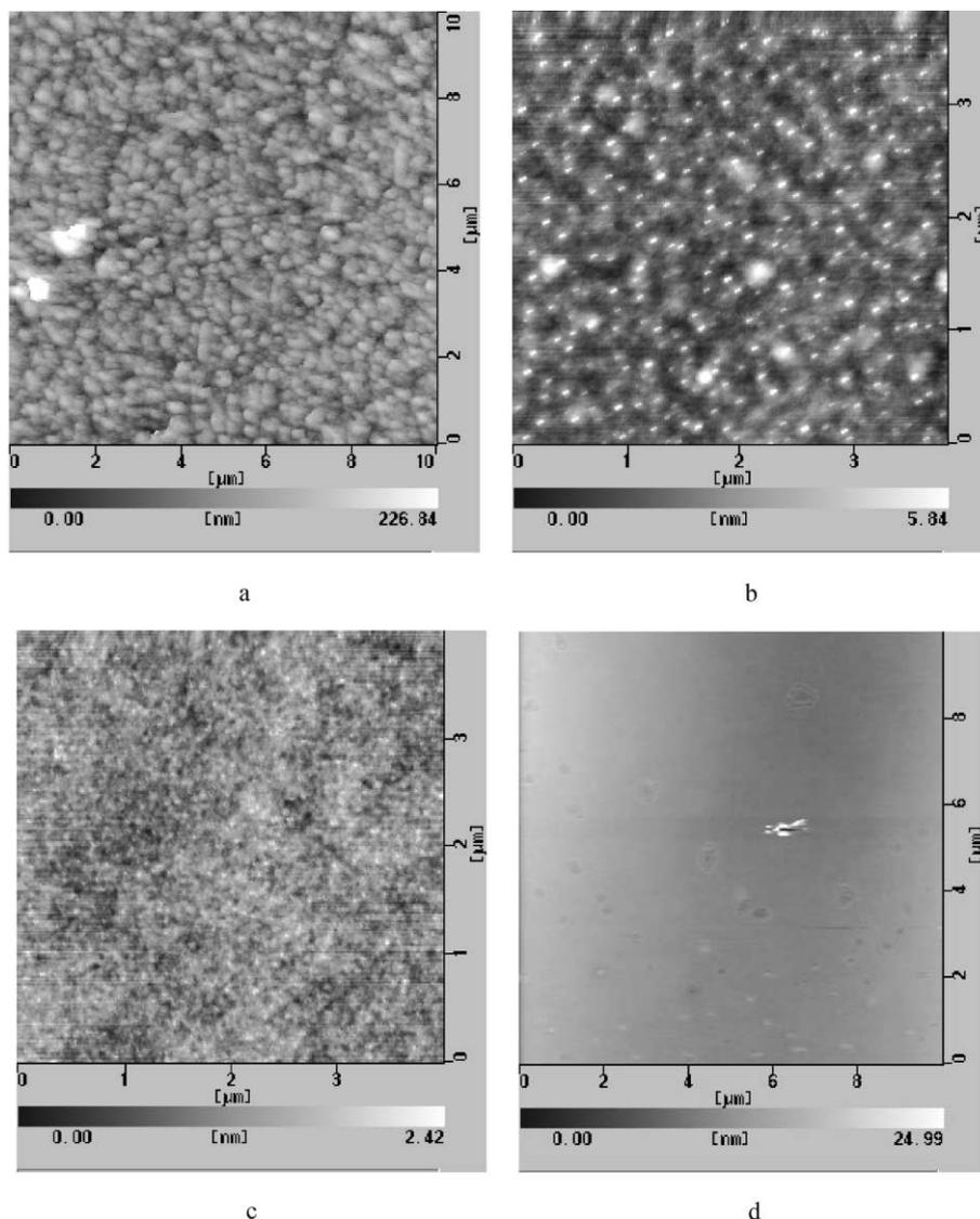
Fig. 4. The AFM photos of D-2 films spin-coated from different pure solvents. (a) methanol; (b) diacetone alcohol; (c) tetrafluoro-propanol; (d) chloroform.
