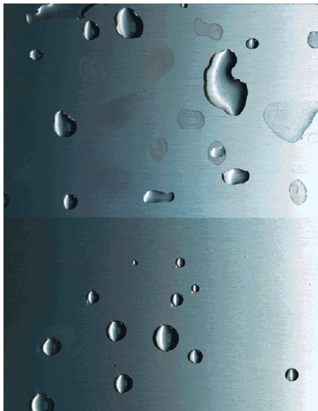
Figure 13. Stainless steel substrate coated by spraying of an abrasion resistant, fluorinated hybrid coating (lower part), demonstrating the "easy-to-clean" aspect (One2Steel, Kuhfuss Sanitär Co., Herford, Germany).
