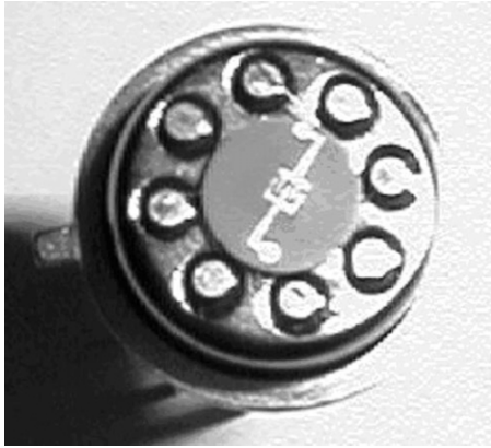
Fig. 1. Investigated sensor in a TO-5 package (without a cap).
