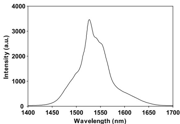
Fig. 6. Near-infrared luminescence spectrum of the glass-ceramics excited by a laser diode at 973 nm.
