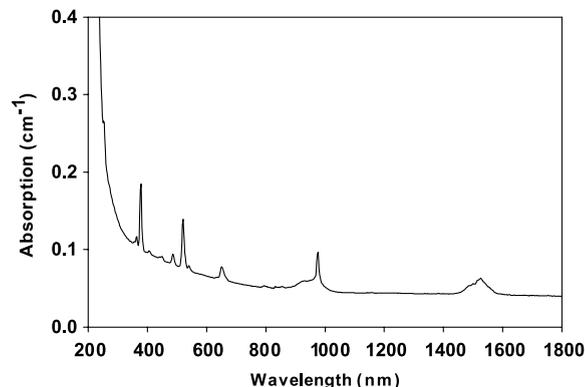
Fig. 2. Optical absorption spectrum of the glass-ceramics sample co-doped with  $\text{Yb}^{3+}$  (0.1 mol%) and  $\text{Er}^{3+}$  (0.1 mol%).
