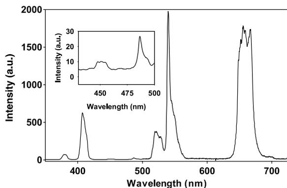
Fig. 3. Upconversion spectrum of the glass-ceramics excited with 973 nm laser diode (inset: magnified spectrum in the wavelength range of 430–500 nm).
