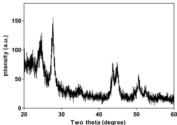
Fig. 5. XRD pattern of the glass-ceramics samples.
