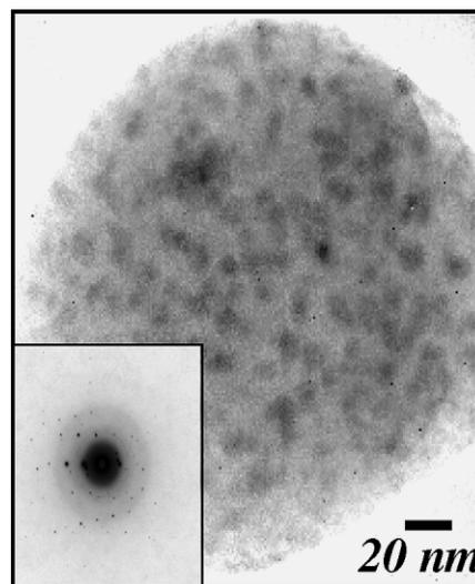
Fig. 4. TEM picture of the sample showing crystalline precipitates. The inset shows the electron diffraction pattern obtained from the precipitated region.
